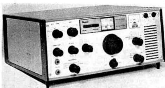
The new Plessey PR155 receiver is fully transistorized and covers 60 kc/s to 30 Mc/s. Short-term stability is better than 5 c/s, and the long-term stability better than 30 c/s on all frequencies.
